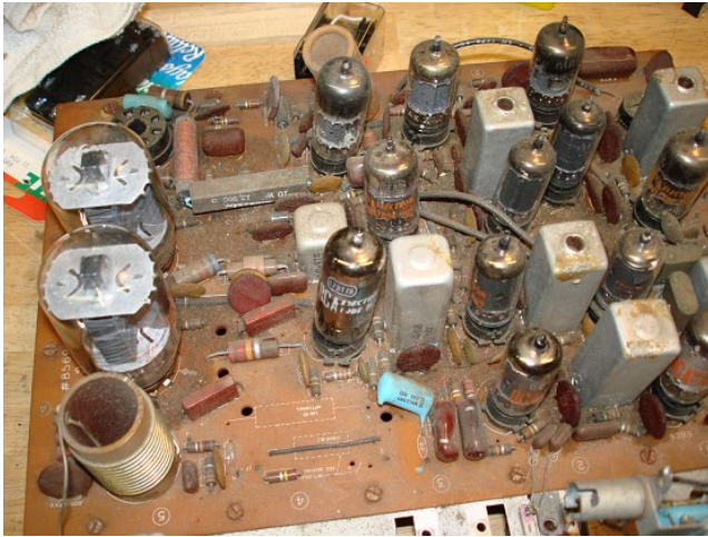
Figure 4 Original Mother Board of HW32A
