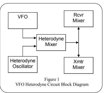
difference frequency is used to produce the 7.20 MHz to 7.30 MHz signal to be transmitted in the 40m band. The transmitted signal can be USB or LSB depending upon the
