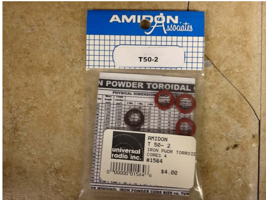
Figure 7 A package of toroids used in the ham bands
