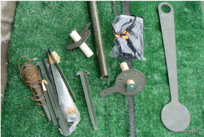
The guy rings were cut from the mast paddles on the right. The 6" x 1-1/2" wood dowel retains the ring when the ring is placed at the top of the mast.
