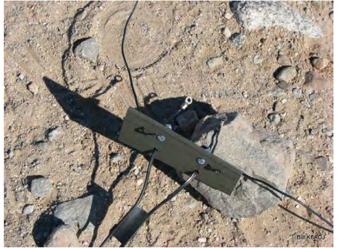
The feed point support is made from the remainder of the green plastic mast paddles. The center support provides strain relieve to the radiator and the feed line. Termination is soldered into stout ring connectors on 8x32 SS hardware.
