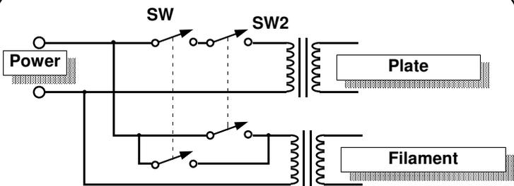
Answer to last month's puzzle. Either switch turns on the filament; both must be closed to turn on the plate. The filament switches form an "OR" circuit. The plate switches form an "AND" circuit.
