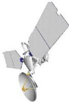
The orbiter's radio operates in the X-band of the radio spectrum, at a frequency of around 8 Gigahertz. The orbiter will also be used as a telecommunications link for future missions.
