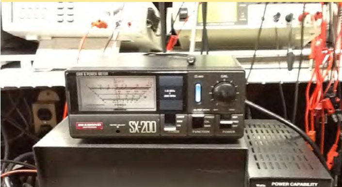
Figure 3: Power Meter Reading 1W Output 3.6MHz
