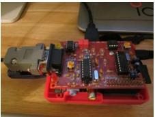
The finished kit is plugged into the GPIO connector on a Raspberry Pi (RPi) which is then attached to a HDMI monitor,
