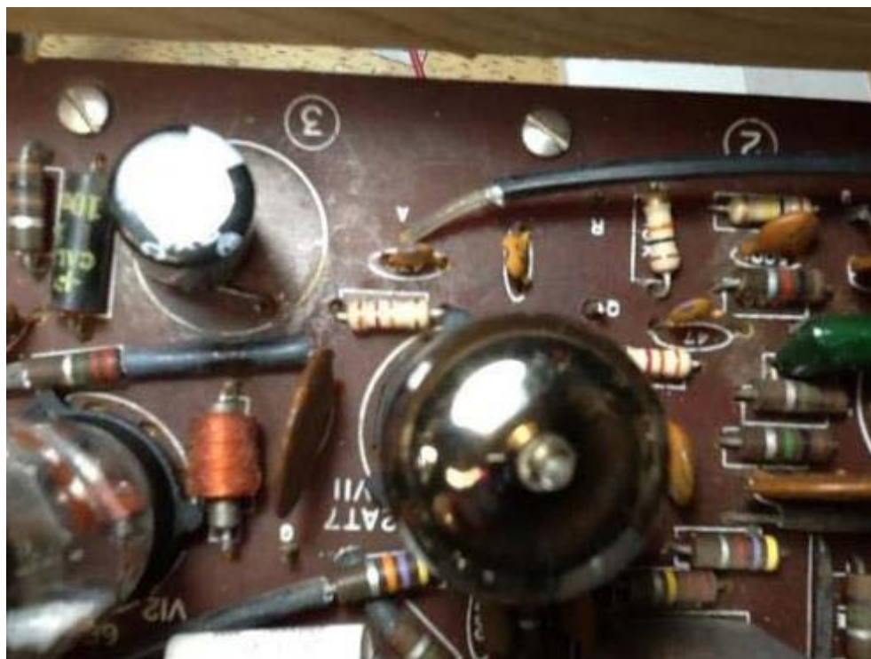
Figure 3 Re-soldered carrier oscillator components
