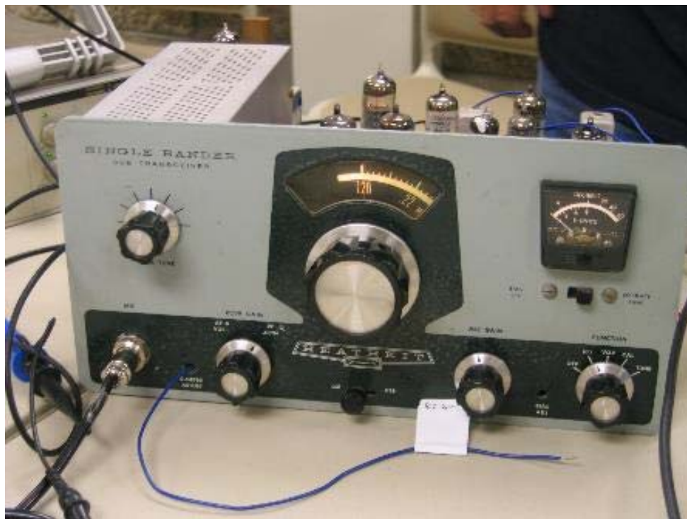
Figure 2 HW22A with cover removed
