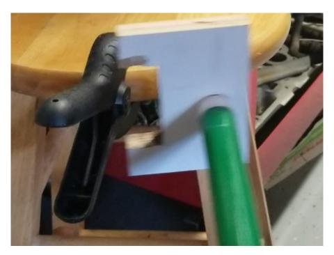
A hefty yank on the clothesline should pull the clamp off the rafter... care should be used to avoid it falling on your head!
