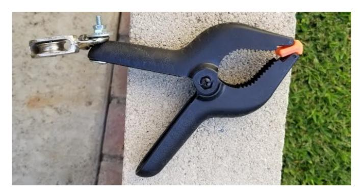
Start by bolting the pulley with clothes line rope loop to one side of the clamp handle. The rope loop needs to be long enough to reach to some feature that will allow you to tie it off when the antenna is hoisted. The rope loop allows the ability to raise and lower for maintenance or experimenting with different designs. Additionally, it allows you to quickly and easily remove the clamp when necessary to satisfy #4 above by giving it a tug to pull the clamp off.
