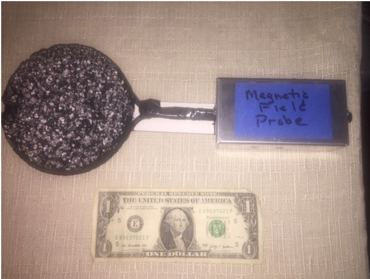
Figure 2. A small magnetic loop probe was used to precisely locate the offending noise source
