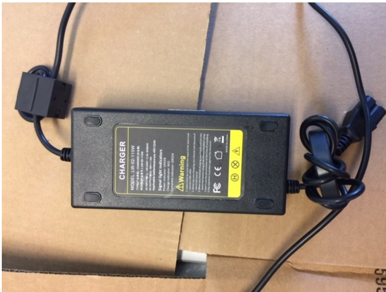
Figure 4. Battery Charger with Input and Output wires wrapped around Ferrite forms
