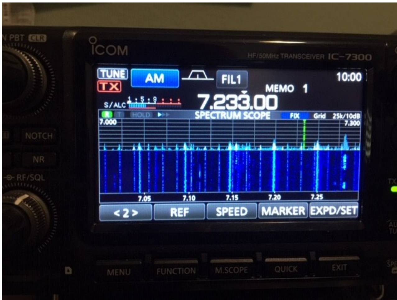
Figure 1. 40 Meter Picket Fence S9 Noise Dominates Band
