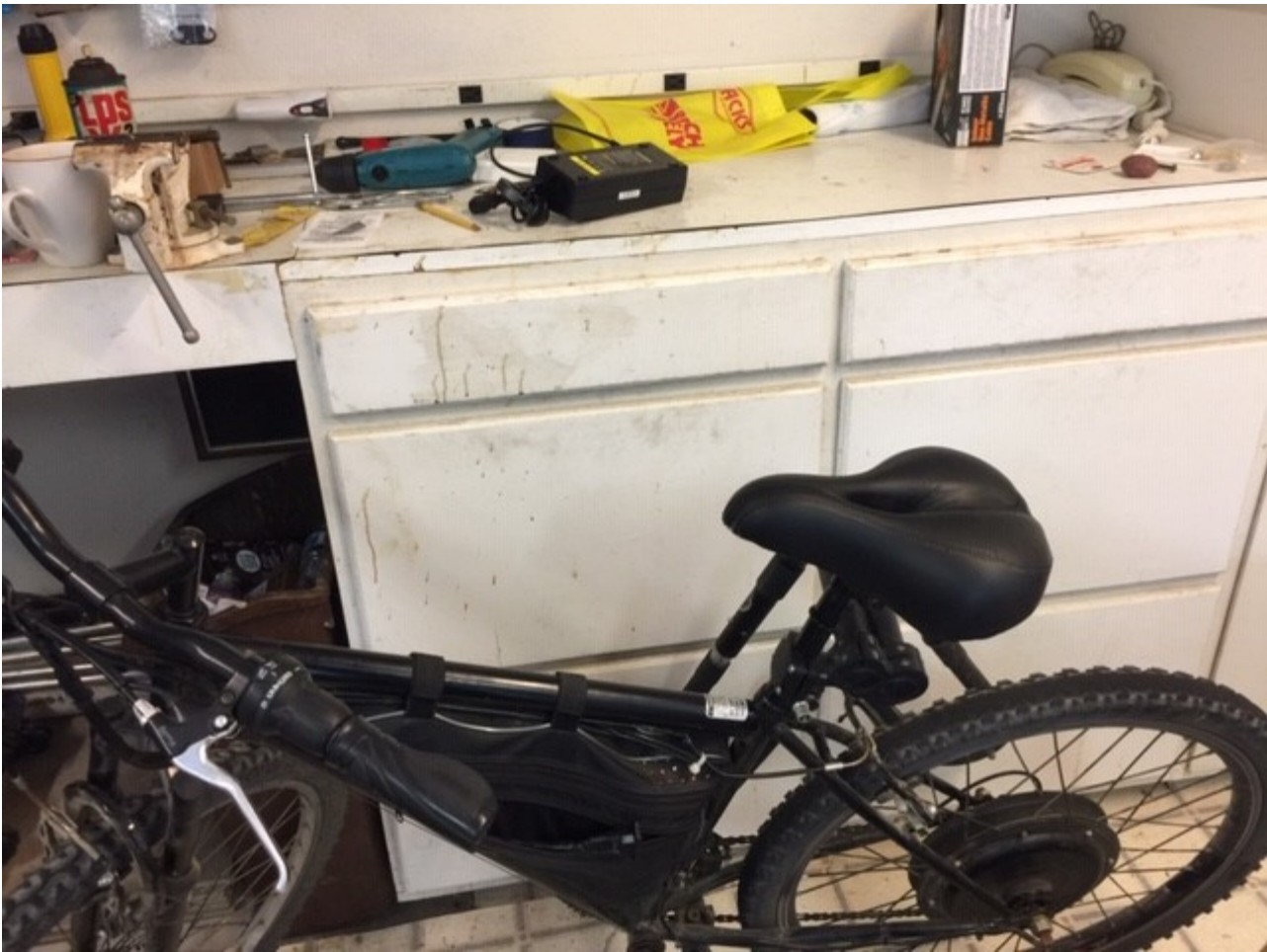
Figure 3. Noise Culprit was E-Bike Li-ion 48 V 12 Ah Battery Charger
