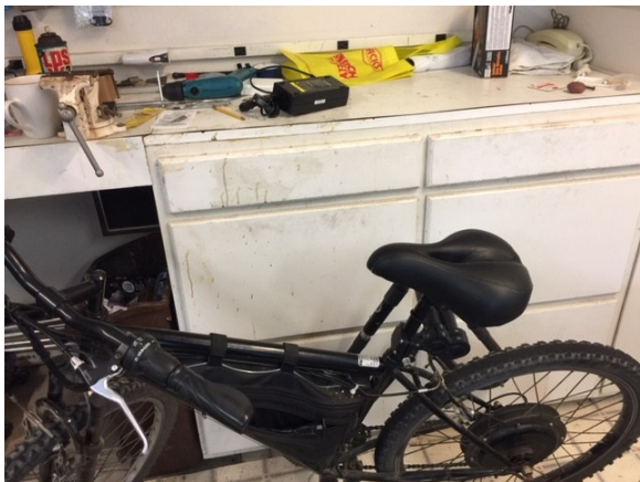
Figure 2. Noise Culprit was E-Bike Li-ion 48 V 12 Ah Battery Charger
