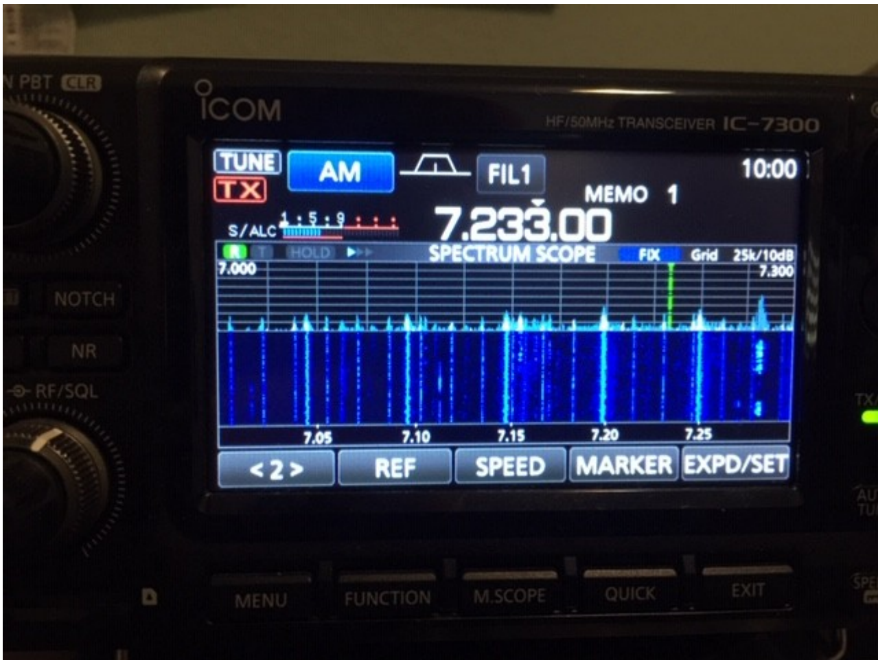
Figure 1. 40 Meter Picket Fence S9 Noise Dominates Band
