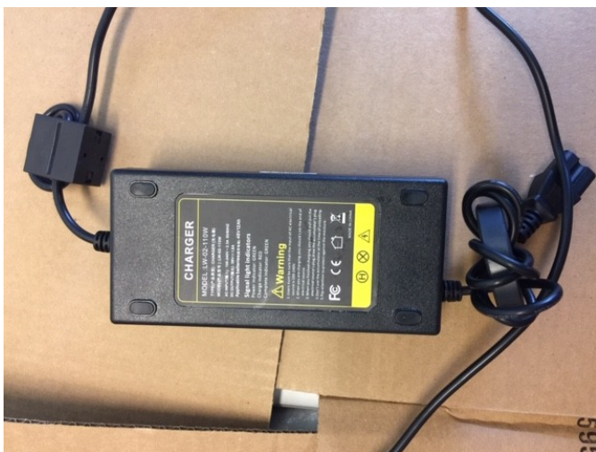
Figure 3. Battery Charger with Input and Output wires wrapped around Ferrite forms
