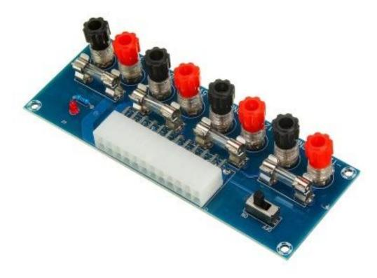
The result is a four output supply great for repairs, development, and experimenting. The four outputs are:
