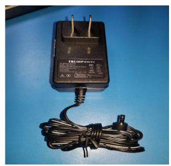
50 Trumpower 4.65V 2.15A supplies with a 3.5mm plug (4.22V @ 2.15A)
