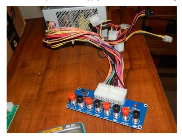
A versatile lab power supply can be assembled from an old ATX supply from a desktop PC. These supplies are available from around \$20 on ebay and \$40 on Amazon. They may be found for next to nothing at swap meets and even free from a friend's garage or junk box.
