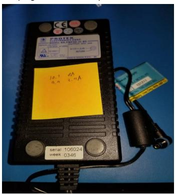
26 Protek 9-11V 3.4A 5.5x2.2mm uses modular power cord(9.9V 3.4A)
