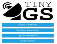
The TinyGS firmware hosts a wireless access point (AP). When first booted, the ESP32 will display the AP SSID and IP address. Connect your computer or tablet to the SSID on the display. Once connected, open a browser and
