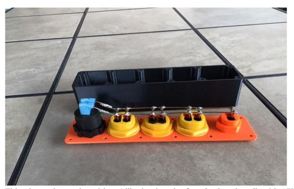
This photo shows the wiring. I like having the fuse in the pig-tail cable. Eliminating the power switch and the external fuse simplifies the wiring. Solder quickly as not to melt plastic. Wiring is more complex if you want an internal fuse and switch. I use Romex wire with the insulation stripped off. Don't nick the wire when stripping off the insulation. If you nick the copper wire, it can easily break in two when bending the wire.
