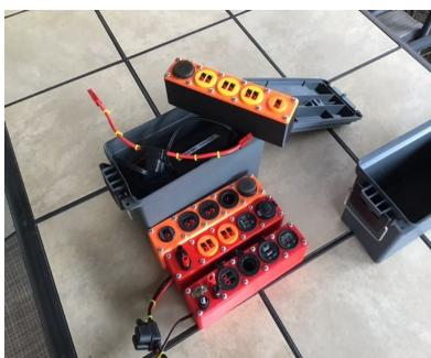
This example illustrates several different configurations of connector boxes. I found the four port design seems to work well. I like having a volt meter. The power switch is not really needed, just unplug the pig-tail connector to turn it off. Options are USB adapters, 12v socket, and powerpoles. There is a combo USB 5V and voltmeter on Amazon somewhere.
