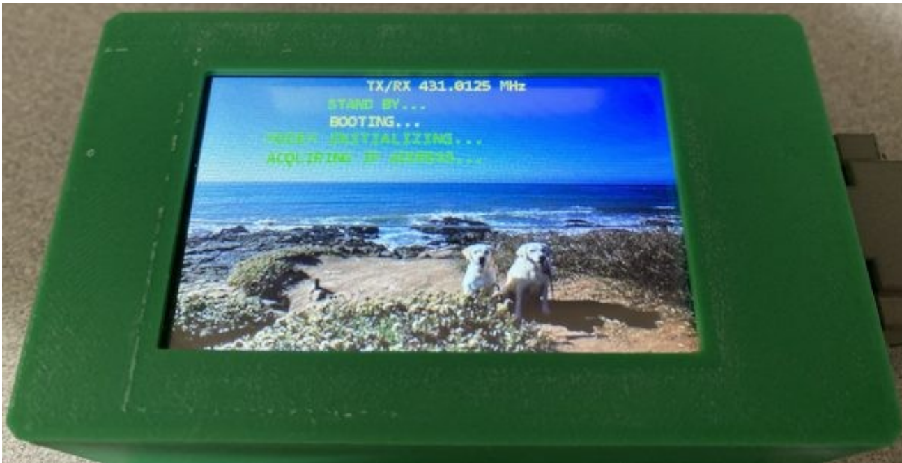
Close up view of the 3D printed enclosure for Nextion, Pi 3A+ and STM32-DVM board
