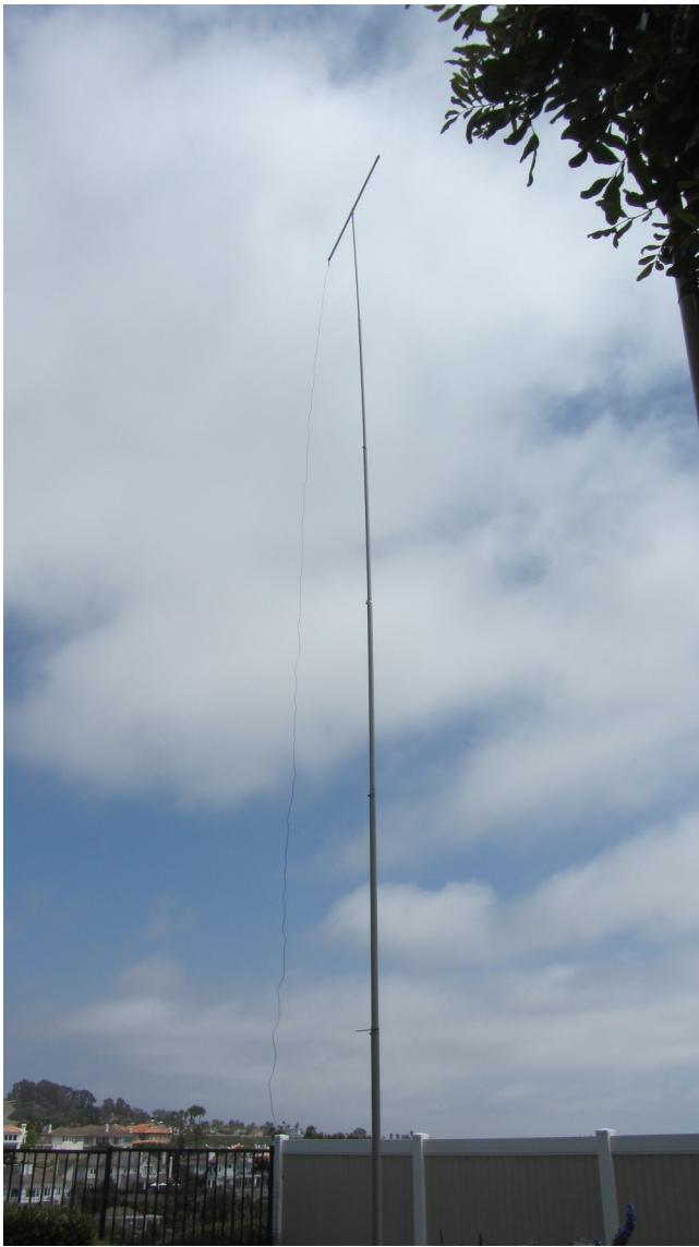
Figure 4 MFJ Pole fully extended, with 40m \frac{1}{4} wave wire, bolted steel pipe base, and a curious bird.
