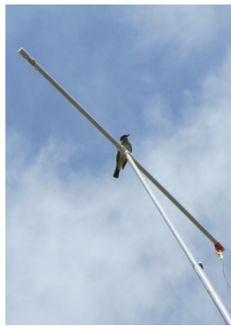
Figure 4 MFJ Pole fully extended, with 40m \frac{1}{4} wave wire, bolted steel pipe base, and a curious bird.
