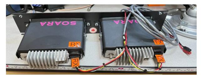
Many years ago, SOARA Repeater and Technical folk fabricated 19" rack shelves that contained Motorola Mitrec radios that were modified for full duplex operation. The shelves were fitted with "flat pack" band reject duplexers and hardline to interconnect them to the radios.
