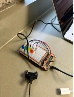
George, KN6OFF demoed APRS decoding with a RTLSDR to turn LEDs on and off. Really cool George.
