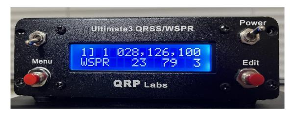
Some time ago I build the Ultimate 3S QRSS/WSPR transmitter from QRP Labs. It came with one low pass filter. I chose the 10meter LPF because I was originally thinking of using the beacon transmitter for the SOARA K6LLL 10 meter CW beacon and the U3S is a great fit for that job. Once I decided to use the transmitter as a WSPR beacon, I needed more bands!
