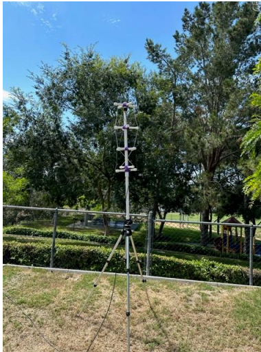
Ed WA6ED demos QFH Antenna to receive NOAA image signals.
