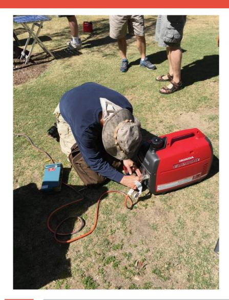
RF noise issues from the generator was fixed in about 30 seconds, Jim, KI6LOM sticking a screwdriver into the ground with a wire to ground generator fixed the noise issue.
